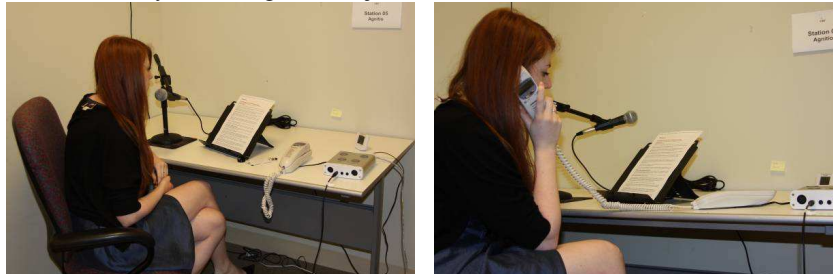
Fig. 1. The setup used to collect audio data corpora for voice biometric modality evaluation.
