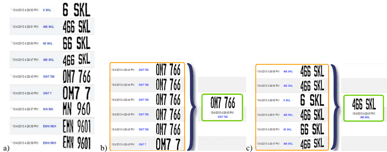
Figure 2. Stream of LPN readings (a) , and the result of LPR data fusion (b,c).
